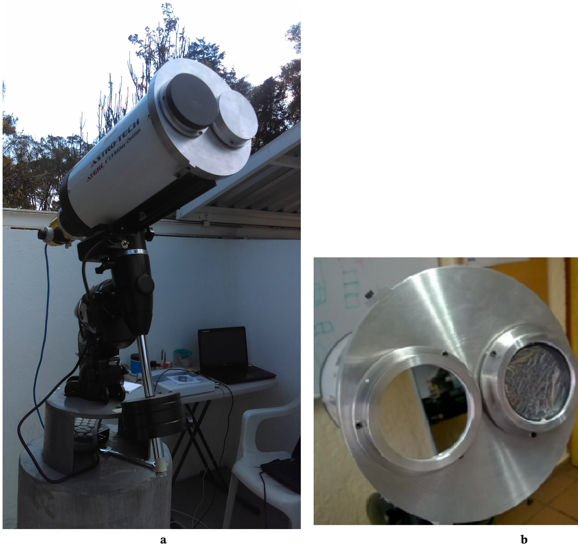
Figure 3. (a) Ritchey-Chretien telescope with the filter cap. (b) Filter cap of the RC telescope. The filter on the left was made of a natural germanium crystal. It has an aperture of 72 mm. The window on the right is for the neutral filter for observing in visible light.
